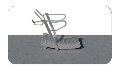
4) Attach the device to the foundation - use 4 M10x100 screws that fit the M14x100 expansion bolts and put on M10 plastic caps.
